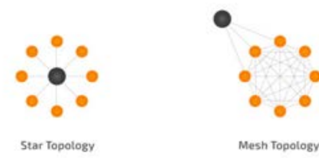
Star topology vs mesh topology
