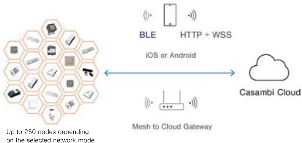
Casambi wireless mesh network with internet gateway
